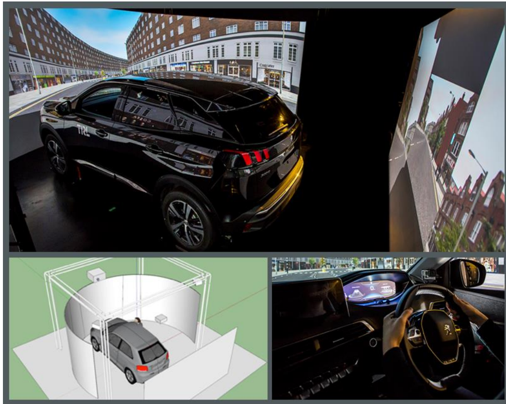
Figure 3: DigiCar, TRL's advanced driving simulator
